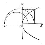
AP and draw PM perpendicular to AX. On BP as a diameter, describe a semi-circumference, and through Q where it intersects the axis AY, draw QM parallel to AX; the point M where it intersects PM, will be a point of the curve. For, from the equation of the circle,
